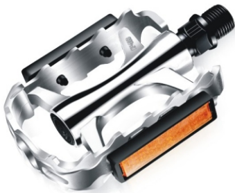
Model:HF-863A MTB Body:Aluminum Barrel polished Bearing:DU bearing Axle:Boron Size:100x80mm Weight:Ball typr 310g/pr
