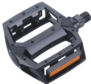
Model:HF-892 MTB/BMX Body:Aluminum Barrel polished Bearing:Ball bearing Axle:Boron Size:108x100mm Weight:Ball typr 446g/pr
