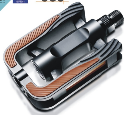
Model:HF-811 COMFORT/CITY Body: 2-Pieces PP body w/inlaid TPR tread Bearing:Ball bearing Axle:Boron Size:105x72mm Weight:Ball typr 307g/pr
