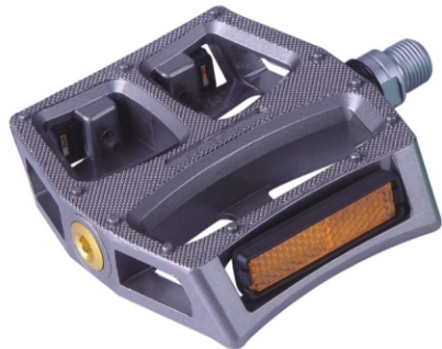
Model:HF-862B FREERIDE/CITY Body:Aluminum Barrel polished/Coating Bearing:Sealed Axle:CR-MO/Boron Size:115x100mm Weight:4Ball typr 496g/pr
