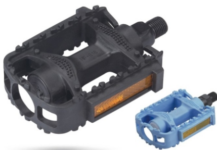
Model: HF-818 CHILDREN'S Body: One-Piece PP Bearing:Ball bearing or W/O Balls Axle:Steel or Boron Size: 100x71mm Weight:Ball typr 256g/pr
