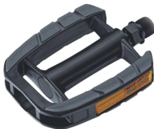
Model:HF-810A COMFORT Body:2-Pieces PP body w/inlaid TPR tread Bearing:DU bearing Axle:Boron Size:100x80mm Weight:Ball typr 240g/pr
