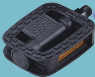
Model:HF-877 COMFORT/CITY Body:One-Piece Black PP Bearing:Ball bearing or W/O balls Axle:Steel or Boron Size:108x75mm Weight:Ball typr 328g/pr
