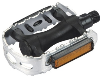
Model:HF-866 MTB Body: Black Nylon Bearing:Ball bearing Axle:Boron Cage:Aluminum Anodized Size:102x80mm Weight:Ball typr 328g/pr
