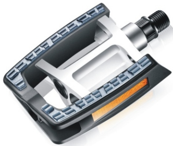
Model:HF-609 COMFORT/CITY Body:Aluminum Barrel polished W/inlaid TPR tread Bearing:DU bearing Axle:Boron Size:110x81mm Weight:Ball typr 333g/pr
