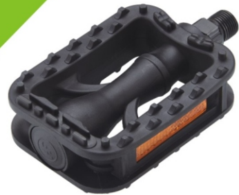
Model:HF-813 COMFORT/CITY Body:One-Piece Black PP Bearing:Ball bearing or W/O balls Axle:Steel or Boron Size:108x72mm Weight:Ball typr 318g/pr
