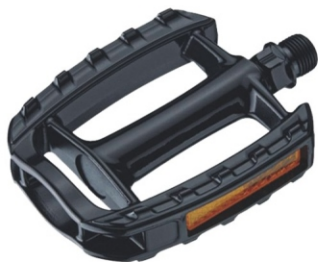
Model:HF-810 COMFORT Body:One-Piece Black PP Bearing:DU bearing Axle:Boron Size:100x80mm Weight:Ball typr 237g/pr
