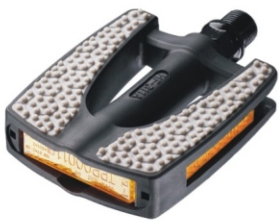
Model:HF-311A CHILDREN'S Body:2-Pieces PP body w/inlaid TPR tread& End Reflector Bearing:DU bearing Axle:Boron Size:96x72mm Weight:Ball typr 250g/pr
