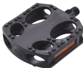
Model:HF-852 MTB/BMX Body:One-Piece Black PP Bearing:Ball bearing Axle:Boron Size:110x105mm Weight:Ball typr 363g/pr
