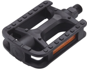
Model:HF-826 COMFORT/CITY Body:One-Piece Black PP Bearing:Ball bearing or W/O balls Axle:Steel or Boron Size:112x78mm Weight:Ball typr 324g/pr
