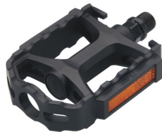
Model:HF-890 COMFORT/CITY Body:One-Piece Black PP Bearing:DU bearing Axle:Boron Size:105x82mm Weight:Ball typr 247g/pr
