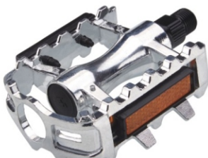
Model:HF-857 MTB Body:Aluminum Barrel polished Bearing:Ball bearing Axle:Boron Size:110x85mm Weight:Ball typr 392g/pr
