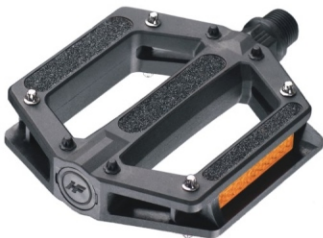
Model:HF-859 MTB/BMX Body:Plastic body W/Sand paper&Pins Bearing:DU bearing Axle:Boron Size:108x91mm Weight:Ball typr 316g/pr
