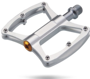
Model:HF-623 FREERIDE Body:Aluminum Extruded/CNC machined Bearing:Sealed/DU Axle:CR-MO/Boron Size:100x101mm Weight:Ball typr 282g/pr
