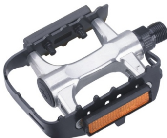
Model:HF-858 MTB Body: Aluminum Barrel polished/Anodized Bearing:Ball bearing Axle:Boron Cage:Aluminum ED Size:100x86mm Weight:Ball typr 346g/pr
