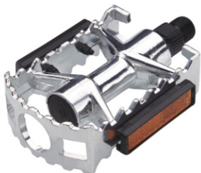
Model:HF-835 MTB Body:Aluminum Barrel polished Bearing:Ball bearing Axle:Boron Size:102x80mm Weight:Ball typr 353g/pr
