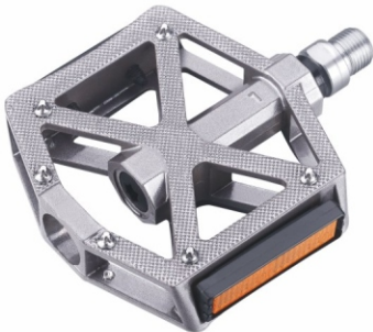
Model:HF-603S MTB/BMX Body:Aluminum Extruded/CNC machined Bearing:Sealed Axle:CR-MO/Boron Size:110x100mm Weight:Ball typr 388g/pr
