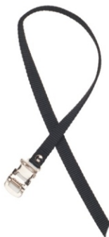
Model:HF-S01 TOE-STRAP 11.5X450mm woven nylon strao Chromeplated steel fastener 50g/pr
