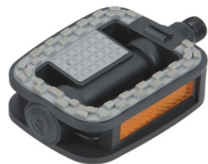
Model:HF-838 COMFORT/CITY Body: 2-Pieces PP body w/inlaid TPR tread Bearing:Ball bearing Axle:Boron Size:110x75mm Weight:Ball typr 375g/pr
