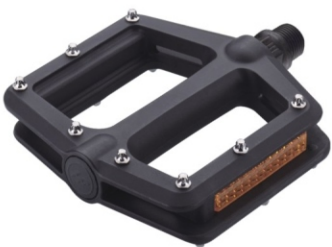
Model:HF-706 MTB/BMX Body:One-Piece Nylon Bearing:DU bearing Axle:Boron Size:110x103mm Weight:Ball typr 344g/pr
