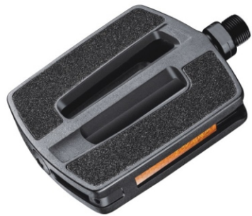
Model:HF-808 COMFORT/CITY Body:Plastic body W/Non-slip Sand tread Bearing:Sealed Axle:Boron Size:110x86mm Weight:Ball typr 333g/pr
