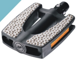
Model:HF-311 CHILDREN'S Body:2-Pieces PP body w/inlaid TPR tread Bearing:DU bearing Axle:Boron Size:96x72mm Weight:Ball typr 268g/pr
