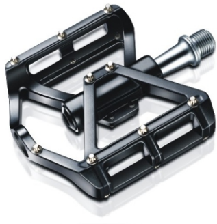
Model:HF-606 BMX Body:Aluminum Extruded/CNC machined Bearing:Sealed/DU Axle:CR-MO/Boron Size:110x100mm Weight:Ball typr 361g/pr
