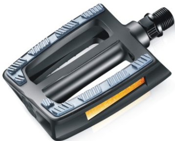
Model:HF-608 COMFORT/CITY Body:2-Pieces PP body w/inlaid TPR tread Bearing:DU bearing Axle:Boron Size:107x81mm Weight:Ball typr 296g/pr
