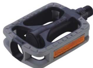
Model:HF-837 COMFORT/CITY Body: 2-Pieces PP body w/inlaid TPR tread Bearing:Ball bearing Axle:Boron Size:105x70mm Weight:Ball typr 297g/pr
