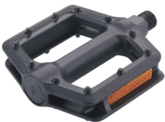
Model:HF-899 MTB/BMX/CITY Body:One-Piece Black PP Bearing:Ball bearing or W/O balls Axle:Boron or Steel Size:108x97mm Weight:Ball typr 298g/pr
